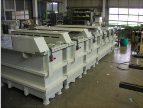
Sedimentation tank with filterpress
