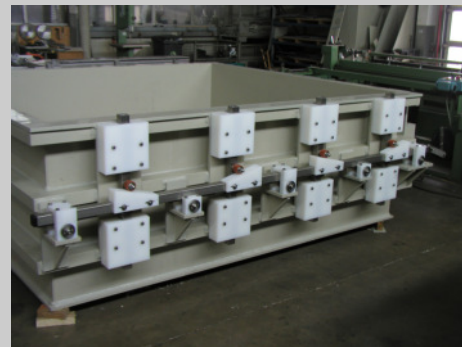
Electroplating tank with goods movement
